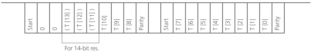
Figure 1.2 – Full ZACwire™ Temperature Transmission from TSic
